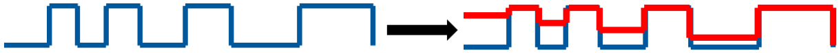
Figure 91: general idea of adaption of the profile depth according to the line density. In principle, the higher line density should give higher efficiency at lower profile depths than the lower line density (see red line on the right).
