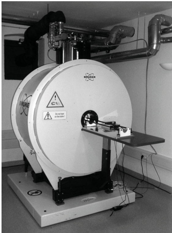
Figure 1. Bruker Pharmascan 70/16 AS. The specimen is inserted into the horizontal bore of the magnet.
