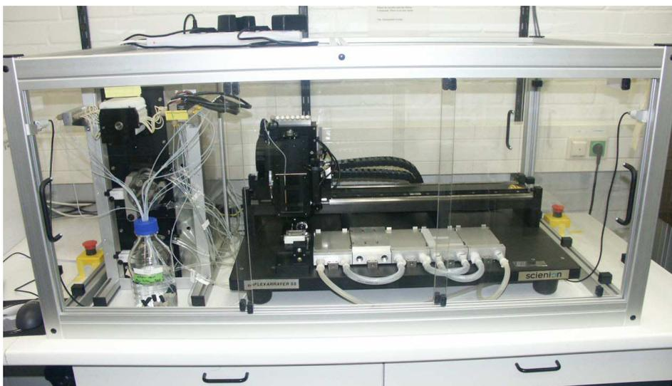
Figure 10: SciFlexArrayer - piezo dispensing station
