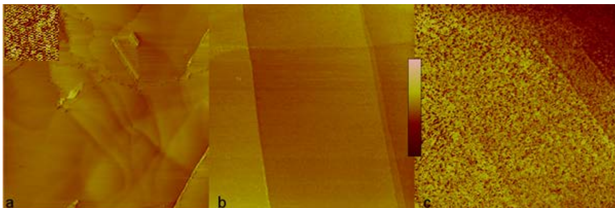
Figure 6.4 STM images of HOPGs (1mmx1mm, I=2\text{nA} ), the height of the scale is 10nm for all three images (a) freshly cleaved HOPG ( U=20\text{mV} ). Inlet: atomic resolved image ( 5\text{nm}\times 5\text{nm} , U=20\text{mV} , I=2\text{nA} ); (b) 500V, 0.1\mu\text{A}\times 3\text{min} ( U=150\text{mV} ); (c) 500V, 0.1\mu\text{A}\times 24\text{min} ( U=150\text{mV} )
