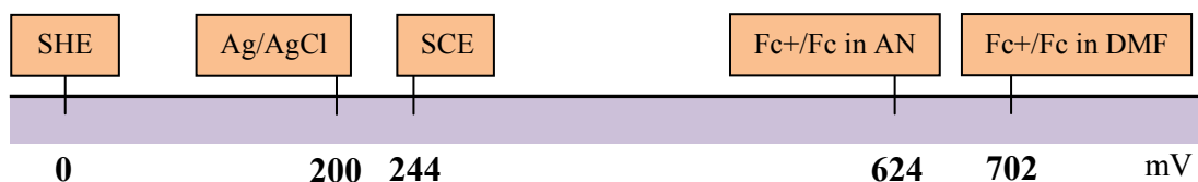
Figure 13. Scale representing the redox potentials of reference electrodes relative SHE
