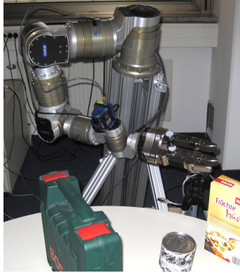
(a) The whole setup: robot, laser sensor and workspace cluttered with various obstacles.
