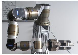
(a) The joints as they look on real Schunk LWA3 hardware with 7 arm joints connecting the arm links.
