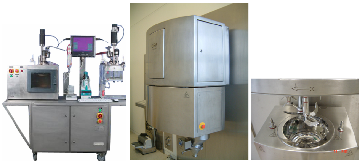
Figure 1.3 Single pot in lab scale (left) and production/pilot scale (right)
