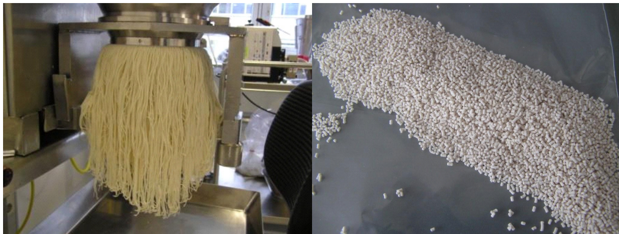
Figure 3.44 Dumbbell shaped pellets formed from long strands during the extrusion process
