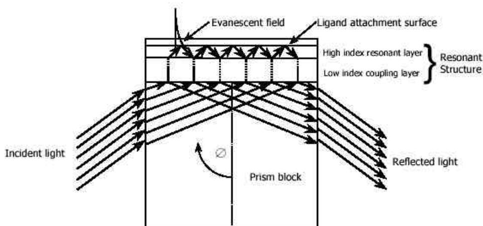
**Fig.7 Configuration of the Resonant Mirror Sensor Device** ([www.Affinity-sensors.com](http://www.Affinity-sensors.com))
