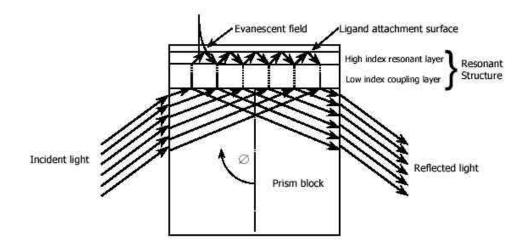
**Fig.7 Configuration of the Resonant Mirror Sensor Device** (www.Affinity-sensors.com) Changes in refractive index at the ligand attachment surface of the device (the biological layer) change the angle at which light can be made to propagate in the waveguide. Laser light (670nm) is scanned at a 10° angle across the device, see Fig. 8.
