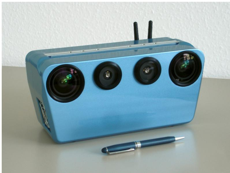
**Figure 6.4:** Sensor head prototype
