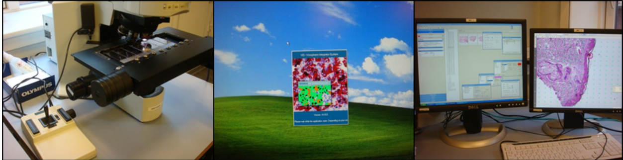
Figure 7. Illustration of the Visiopharm NewCast software v. 4.4.5.0 connected to Olympus BX51 light microscope with a motorised Prior stage with spacing for 8 slides.
