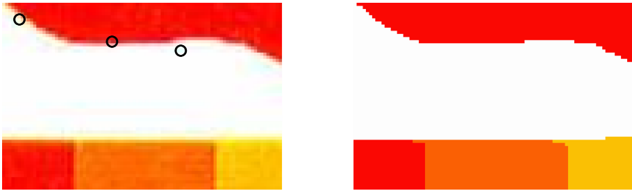
Figure 2.4. Segmentation—trademark image I: original (left) and segmented (right) 90 \times 60 pixel detail of a 510 \times 1856 pixel trademark image. The average RGB values of the red region in the upper part are (250, 8, 3) whereas the boundary pixels marked by the black circles have RGB values (255, 255, 222) , (192, 43, 45) , and (227, 255, 252) , respectively.
