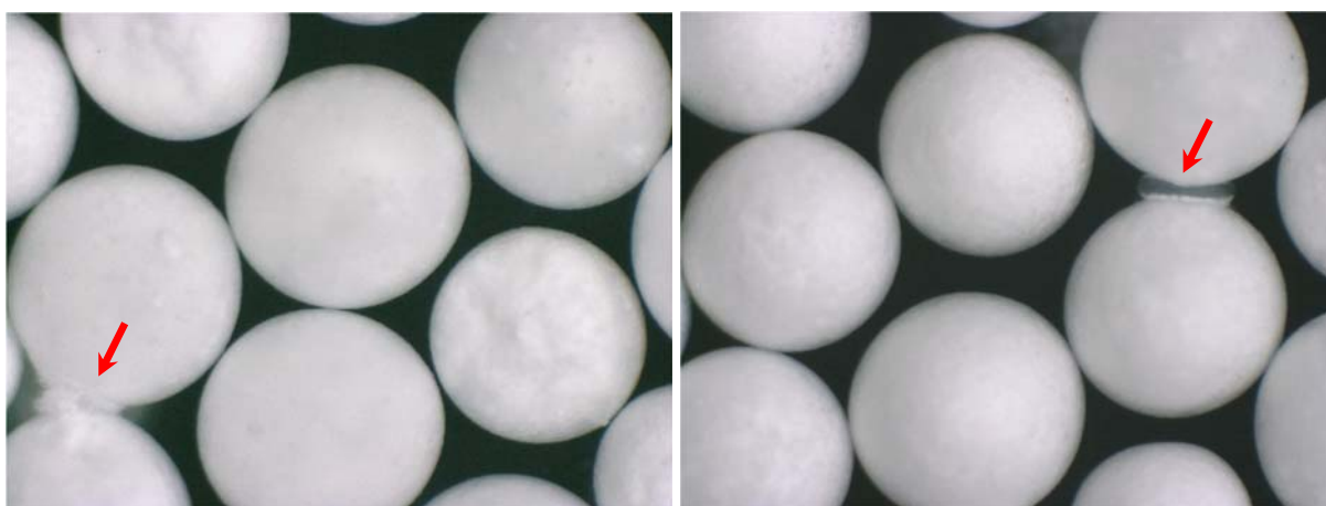
Figure 52. Exemplary pictures of micro-cracking for 50-CBZ-MCC-65:35 during release; solid carbamazepine expelled from minute cracks as white ‘drug powder clouds’
