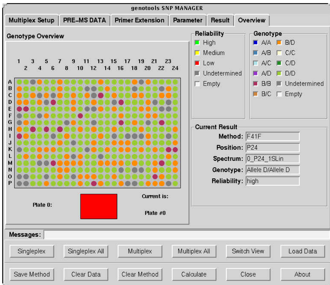
Figure 2.3. Genotype analysis of the results shown in figure 2.2. Again, grey points are undetermined results, while green points stand for homozygote D/D, orange points for heterozygotes B/D and violet points for homozygous B/B DNA. The corresponding biological alleles are thus coded A, B, C, and D.
