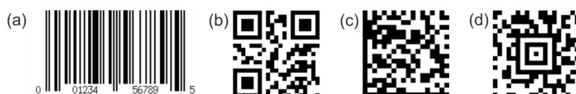
Figure 1.18 Different 1- and 2D barcode types. UPC with encoded information: 001234567895 (a), QR code (b), Data Matrix code (c) and Aztec code (d). All 2D codes have the encoded information: http://www.bam.de .
