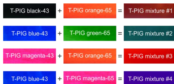
Figure 6.13 Solvent cast PEU films containing 20 wt% of one sort of T-PIG with a CST of 43 °C (left column), 20 wt% of another sort of T-PIG with a CST of 65 °C (column in the middle) and 1:1 mixtures of both (right column). The films had uniform thicknesses of (65 \pm 5) \mu\text{m} . The images were recorded at 23 °C.
