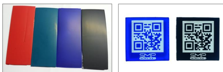
Figure 7.1 Left: PEU plaques solvent cast with PEU pastes containing 20 wt% of Igrazin-red DPP BO, Cobalt chromite green, ultramarine blue and graphite powder ( pigment green 26 ); right: QR code carriers prepared from the blue and black colored PEU plates shown next to it.
