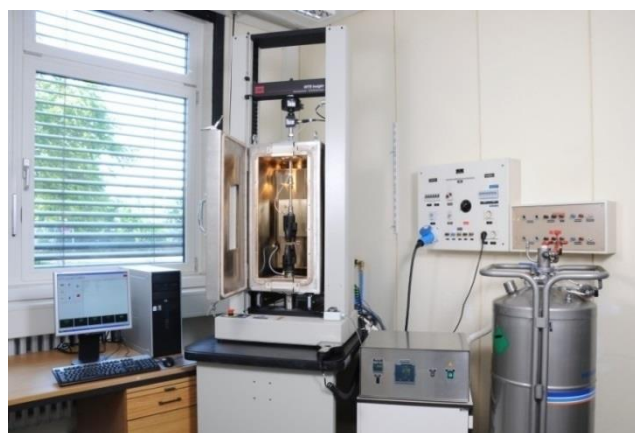
Figure 1.10 MTS tensile testing machine equipped with a thermo-chamber.
