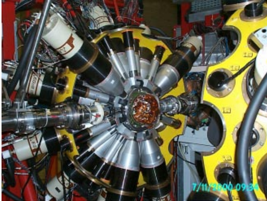
Figure 2.3: A picture of the \gamma -ray detector array GASP. The second half is moved away. In the centre is the silicon detector ball ISIS.
