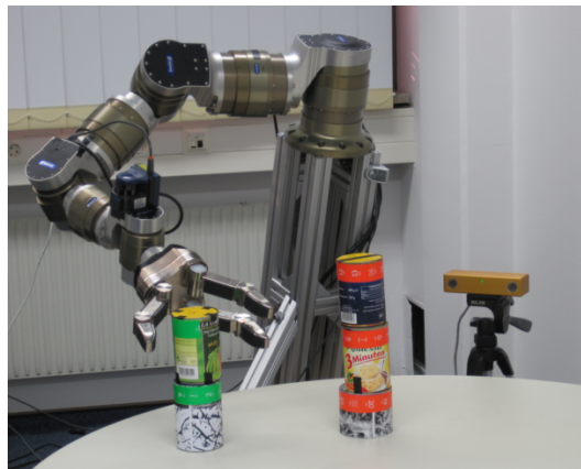
Figure 4.13: The robot has successfully put objects with green and red labels into separate piles, using probabilistic inference on different levels of abstraction for planning and control.
