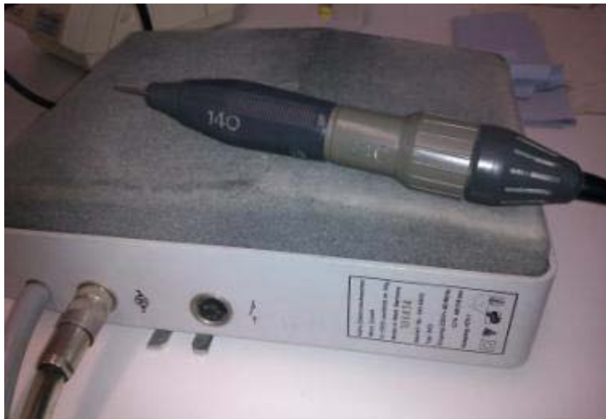
Figure 6: Dental driller which is used for shell sampling. The rotation speed can be regulated by foot.
