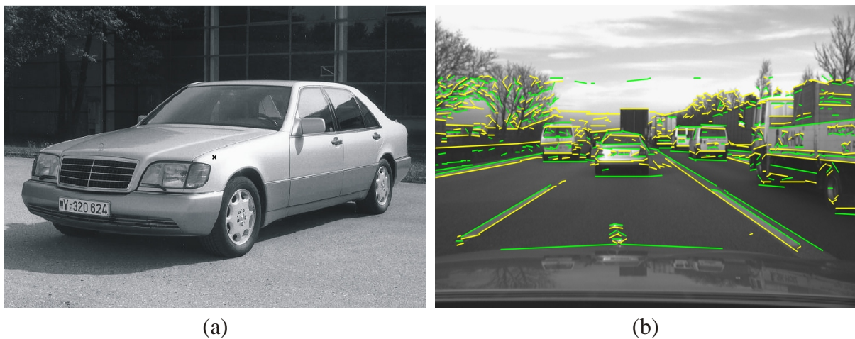
Figure 2.6: (a) The VaMP, Mercedes 500 SEL of the University of the Federal Armed Forces Munich, Germany. It is equipped with four video cameras, a millimeter wave RADAR and eight microprocessors for object recognition and autonomous vehicle guidance. (b) Linking profiles of similar gray values, hypothesis for objects are created. Once the hypotheses exist, tracking is based on the system dynamics approach using motion models of the objects. (with kind permission from Prof. E. D. Dickmanns)
