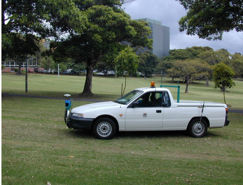
Figure 2.2: At the Australian Center for Field Robotics (ACFR) a utility vehicle is equipped with a laser range scanner for navigation in a park-like environment. Here, the focus of research is on Simultaneous Localization and Map Building (SLAM) algorithms. (with kind permission from Dr. E. M. Nebot)
