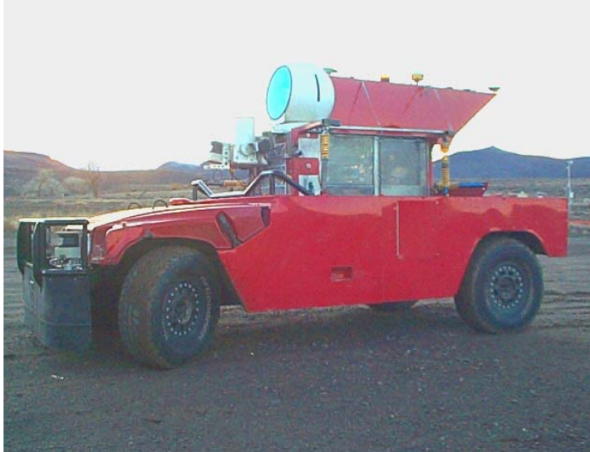
Figure 2.3: The Carnegie Mellon University team’s race vehicle, Sandstorm, is a M998 HMMWV vehicle modified for autonomous race driving. It uses three SICK and one RIEDL laser range scanner, primarily for obstacle detection. (with kind permission from Prof. William L. “Red” Whittaker)
