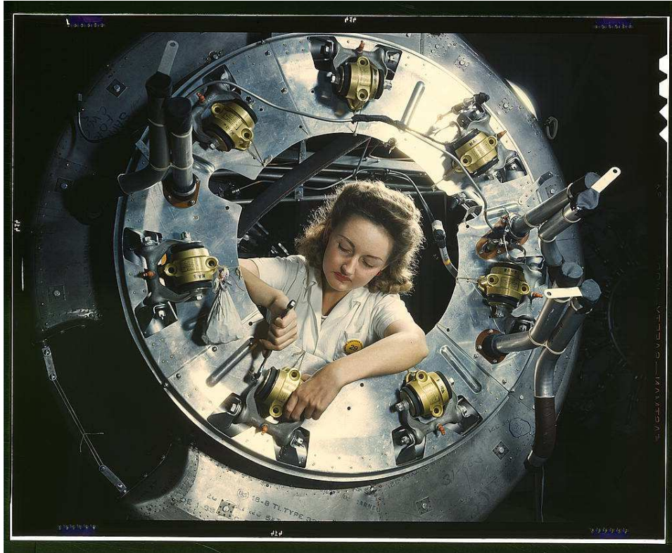
Figure A.3: A. Palmer, “Part of the cowling for one of the motors for a B-25 bomber is assembled in the engine department of North American [Aviation Inc.]’s Inglewood, Calif., plant.” (October 1942). Made for the Office of War Information. Library of Congress, Prints and Photographs Division [reproduction number LC-USW361-453 (35 mm color slide)].
