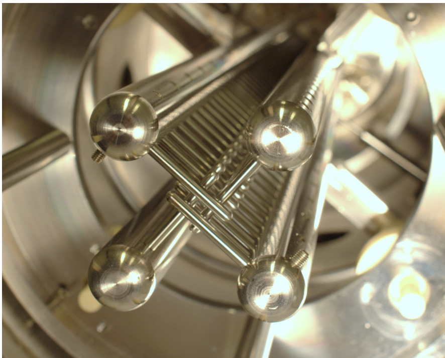
Figure 4.5: Photograph of the 52 cm long, 94-stage Stark decelerator in the vacuum chamber. The point of view is from the back of the Stark decelerator. The steel electrodes have a diameter of 3 mm. The gap within the parallel pairs is 2 mm. The pathway of the molecules points right through the center of the square formed by the adjacent electrode pairs.
