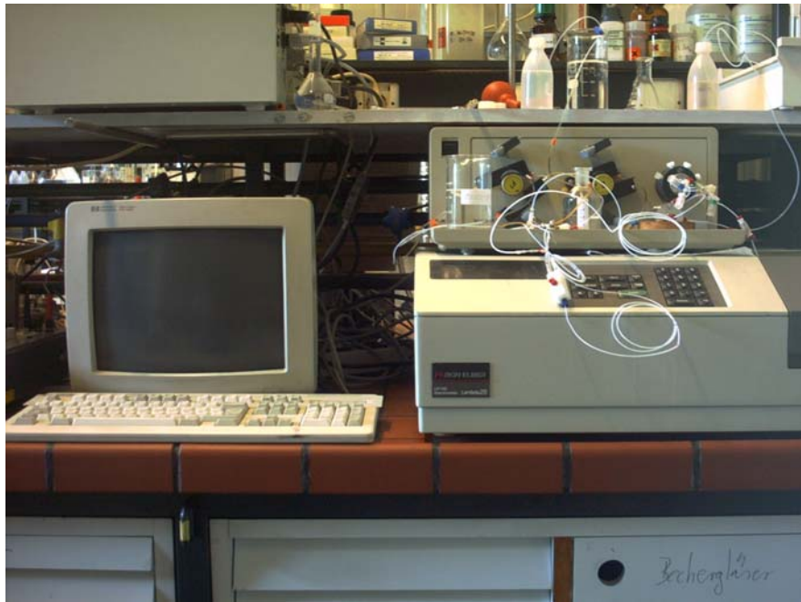
Abb. 4-24: UV/VIS-Spektralphotometer Lambda 2 (Perkin-Elmer)
