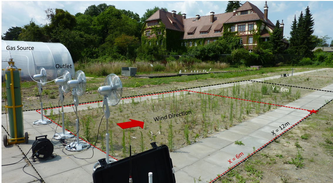
Figure 7.6: Experiment environment and setup of the experiments performed in the Botanical Garden of Berlin. The starting point is indicated by the red star. The red arrow illustrates the main wind direction during the experiments. The rectangular area marked with the red dashed line shows the experiment area of 6 \times 6m^2 , whereas the rectangular area marked with the black dashed line shows the 12 \times 6m^2 experiment area.
