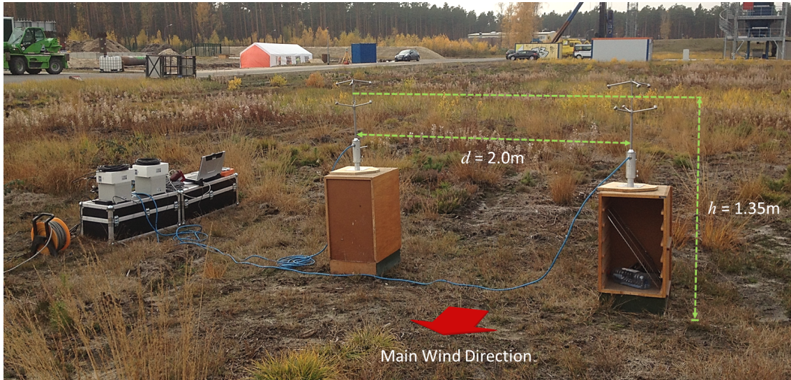
Figure 6.3: Experiment setup to ascertain to which degree the assumption of a uniform wind field holds in a realistic scenario.
