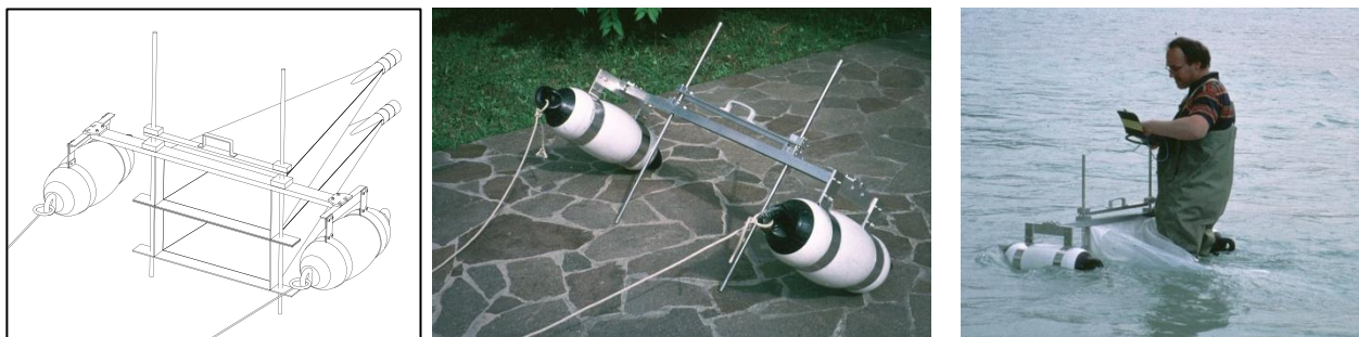
Fig. 5. Example of a sampler to collect FOM and its deployment (source: S.D. Langhans)
