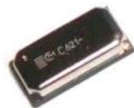
Abbildung 15 1D Gyroskop ENC-03 [Mura11]
