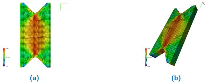
**Figure A.4:** Shear specimen. Color-coding according to the von Mises stress.
