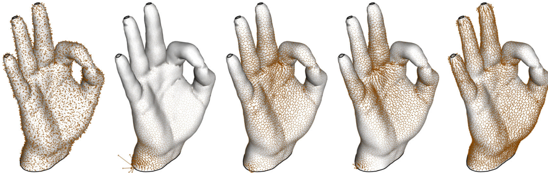
Figure 5.13: Eigenvectors for the next five smallest eigenvalues. These eigenvalues are of orders 10^{-7} to 10^{-3} , whereas the five correct solutions in Figure 5.4 correspond to eigenvalues of order 10^{-16} , so there is a clear gap of magnitude in the eigenspectrum, cf. Table 5.6. Whereas some of these eigenvectors are obviously nonsense (first two images), others can give surprisingly well-structured vector fields, depending on the solver.
