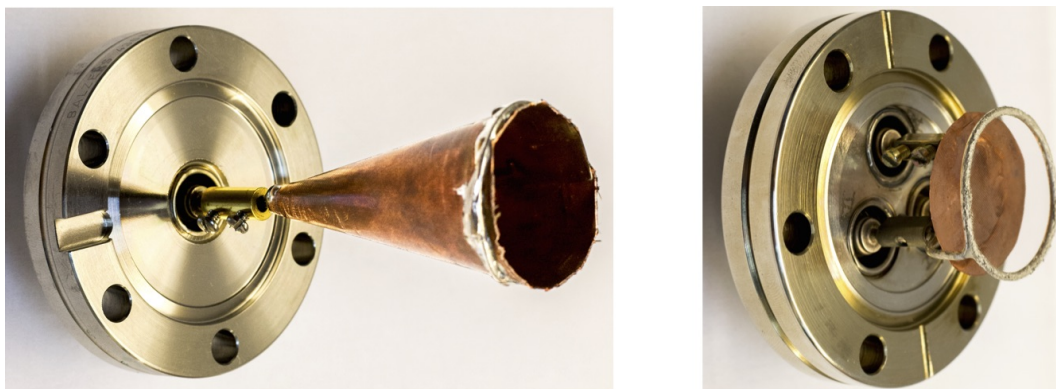
Figure 3.10: Two Faraday cups with a conical and a flat detection surface, respectively, were used in this thesis to detect ion-doped helium droplets.
