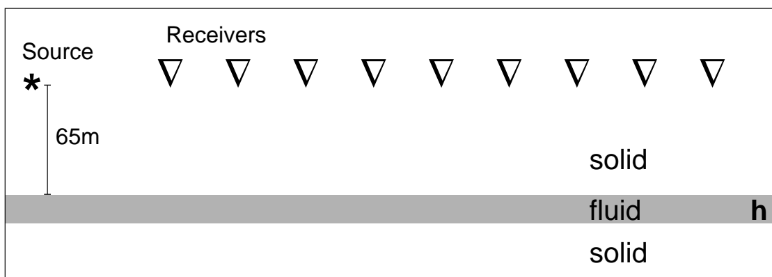
Figure 3.5: Model to obtain angle dependent reflection coefficients using an explosion source.
