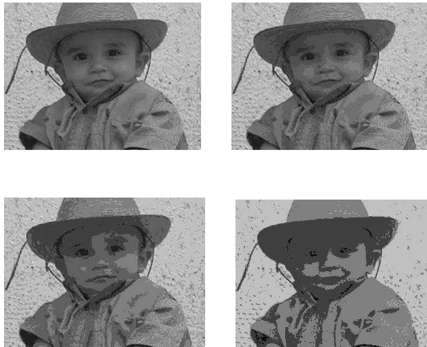
Figure 2.4: An image shown at many different gray level resolutions. Top left: Original image sampled at 256 gray levels. Top right: 64 gray levels. Bottom left: 32 gray levels. Bottom right: 8 gray levels.
