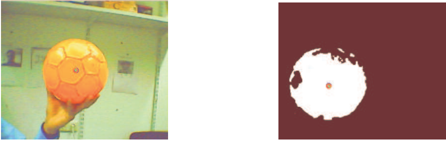
Figure 2.11: A soccer ball image and its resulting binary image with their respective centroid. Left : Original image. Right : calculated centroid.
