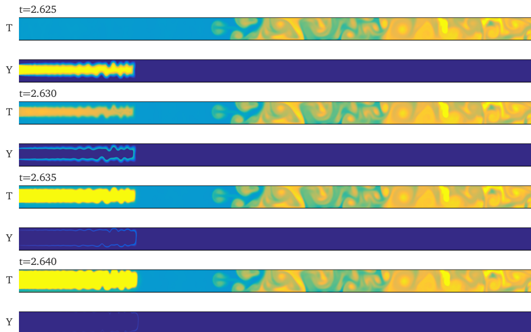
Figure 4.2.14.: Temperatures in a H 2 -SEC with injection at multiple axial positions. Injection may be observed through the temperature drop due to the injected fuel having a lower temperature than the air.
