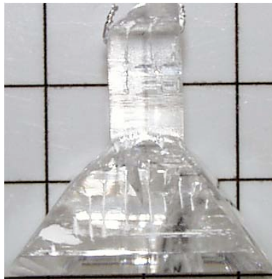
Figure 4.8: Segmented grown Yb:KYW/KYW crystal. The top, undoped KYW segment is grown first. The second KYW segment is 13 at. % Yb-doped. Scale grid: 10 mm. Obtained from FEE GmbH, Germany.
