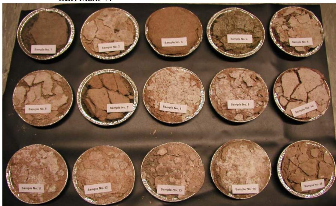
Appendix C: Photographs of saline soil samples which were measured their reflectance spectra by the Infrared Intelligent Spectroradiometer (IRIS)-GER Mark V.
