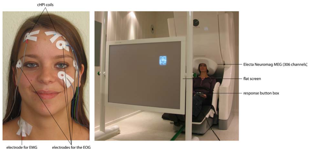
Fig.4: (left) Two pairs of electrodes recorded vertical and horizontal bipolar electrooculograms (EOG). Five continuous head position indicator (cHPI) coils, two placed on the auricles (not visible here), three on the forehead (only two visible here), recorded the subjects' head positions. (right) Electromagnetically shielded room with the 306 channel Vectorview MEG, the back projection screen, and a subject holding the response button box.
