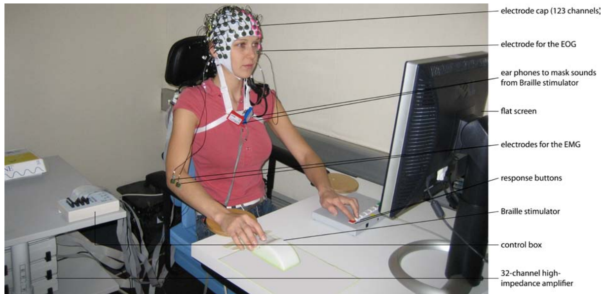
Fig.17: Experimental setup. The subject was seated in an electrically and acoustically shielded room in front of a flat screen. The index finger of the right hand was placed on the Braille stimulator, and the index and the middle fingers of the left hand were placed on the response buttons. The 123-channel electrode cap and the additional five electrodes to record electrooculogram (EOG) and electromyogram (EMG) were joined in a control box which in turn was connected to four 32-channel high-impedance amplifiers (for detailed description, see text). The signal was then relayed to a laptop for data acquisition (not visible here).
