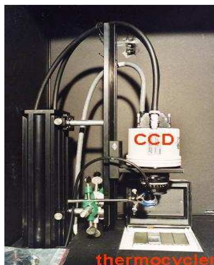
Figure 8. CCD camera with high sensitivity for fluorescence detection.
