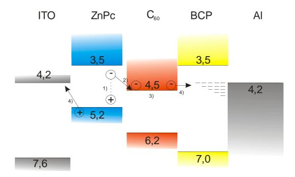
Figure 2. Energy level diagram of the ITO/ZnPc/ $C_{60}$ /BCP/Al cell; Values in eV. Process 1) stands for exciton creation in absorber layer; process 2) is charge separation on ZnPc- $C_{60}$  interface; process 3) is the diffusion of charges; process 4) is charge transfer to contacts through the buffer layers. Work function of ITO can vary up to 4,7 eV, but 4,2 eV is the value, measured on a clean-sputtered ITO surface
