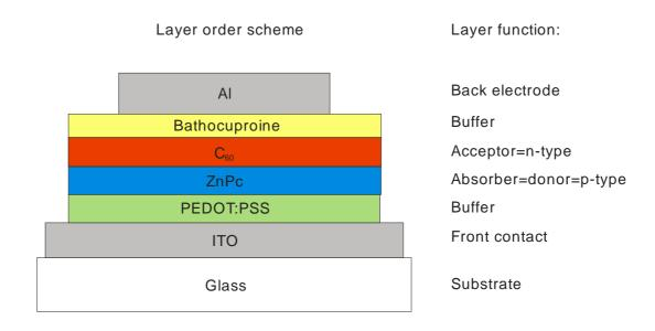
Figure 1.  $ZnPc/C_{60}$  solar cell architecture. The two active layers ZnPc and  $C_{60}$  are sandwiched between the two buffers, which lay next to the electrodes
