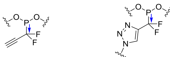
Figure 6.2: Strong electron-withdrawing groups next to the phosphorus ought to reduce the tendency of phosphonites to be hydrolysed.
