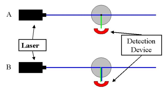
Figure 61: Principle of the fluorescence spectrometer. A displays the case for the measurement of fluorescence and B displays the scattering of the laser beam by particles in the solution
