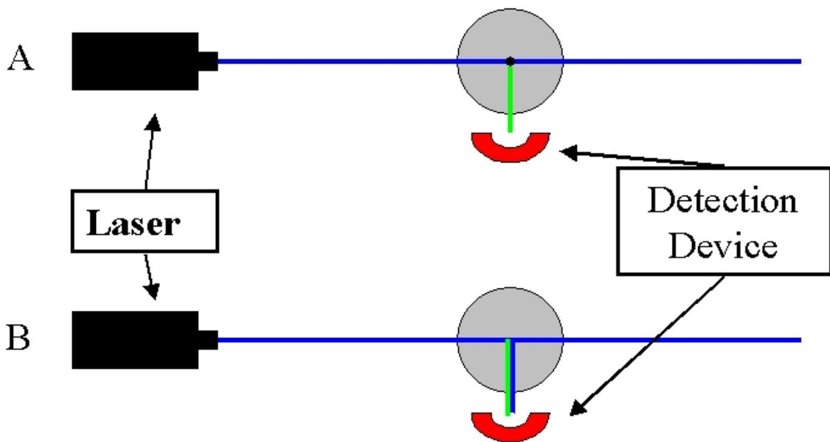
**Figure 61: Principle of the fluorescence spectrometer. A displays the case for the measurement of fluorescence and B displays the scattering of the laser beam by particles in the solution**
