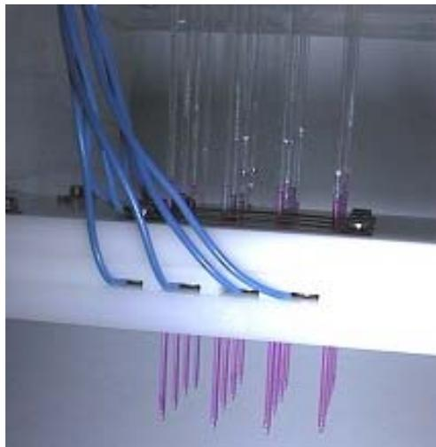
**Figure 4: Spotting head with 16 piezoelectric nozzles (courtesy of Dr. L. Nyarsik, MPIMG)**
