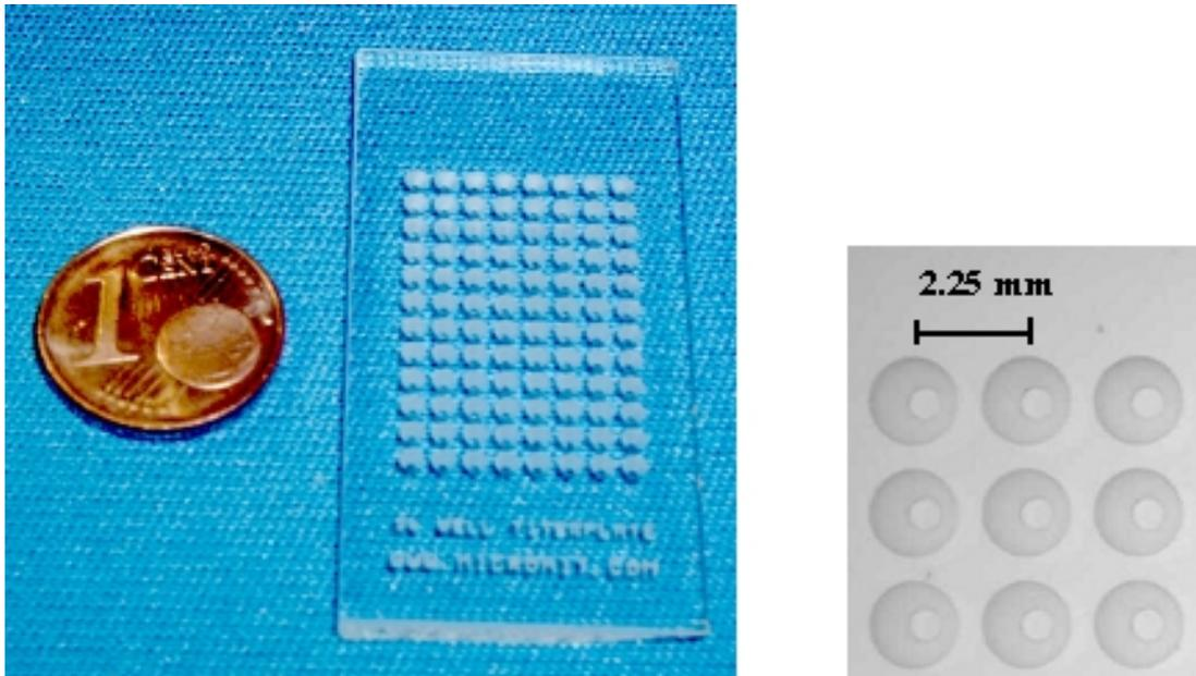
**Figure 7: Left: Photograph of the nanowell plate comprising 12x8 wells with a well volume of 1.5  $\mu$ l. Right: Enlarged photograph of the nanowells with a spacing of 2.25 mm between each well**
