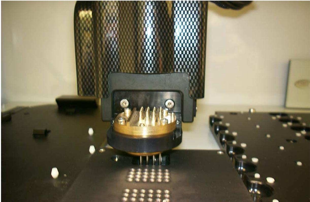
**Figure 3: Spotting head with 16 solid steel pins**
