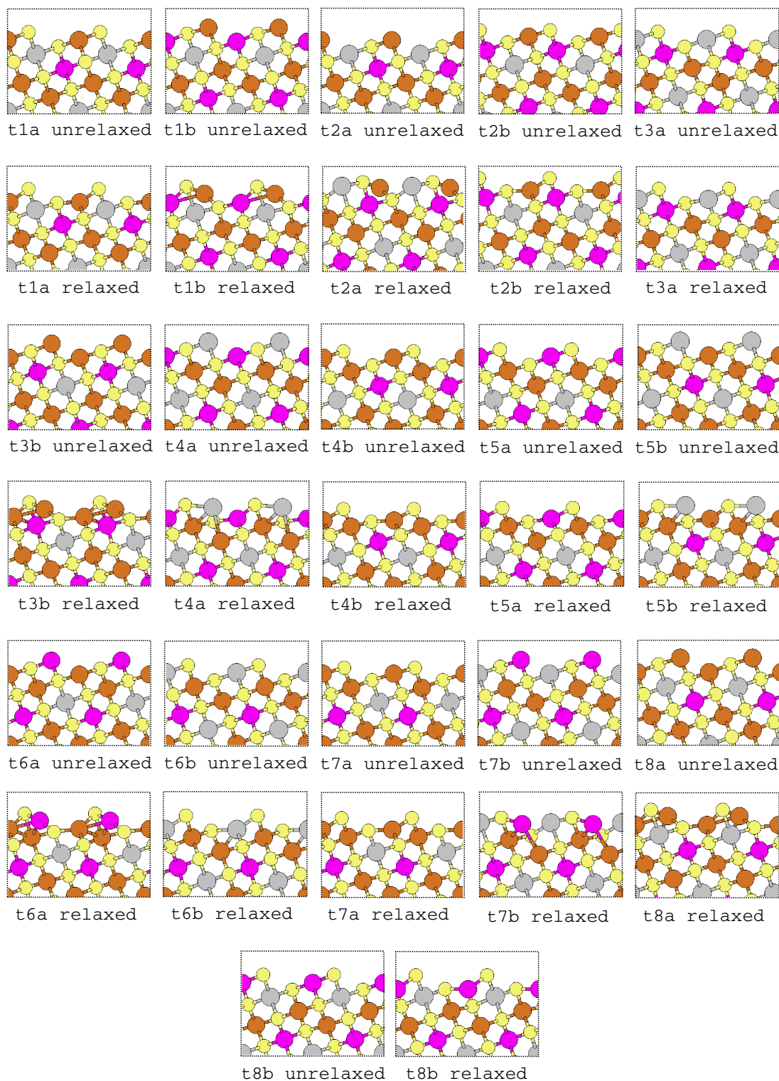
Figure 4.7: Unrelaxed and relaxed terminations of the (101) surface of CZTS at the PBE-level. Zn is shown in pink, Cu in brown, Sn in gray and S in yellow.
