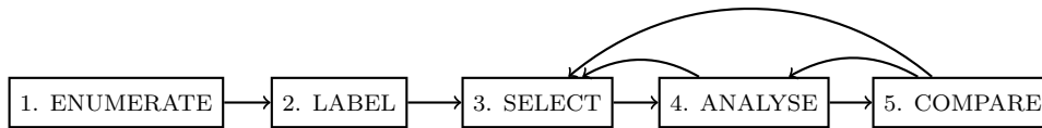
Figure 1.2: Our workflow starts with the enumeration (1) of all possible models that fit the expectations of the modeller about the structure. Each of the models is evaluated for certain properties (2) like dynamical behaviour, and the result of the evaluation is stored with the model as its label . After the models are labelled, the user can select (3) a subset of these that seem of special interest. This selection can then be analysed using various tools (4) and compared to other selections (5). The selection or analysis can then be refined based on the newly gained knowledge.
