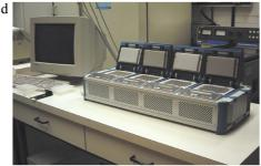
Figure 8. Pictures of the Genesis Workstation 200 from Tecan (a), the automatic incubator cytomat 6002 from Heraeus (b, c), and the PrimusHT multiblock thermal cyclers from MWG Biotech (d), which were used to handle and amplify the cDNA clones for the microarray.
