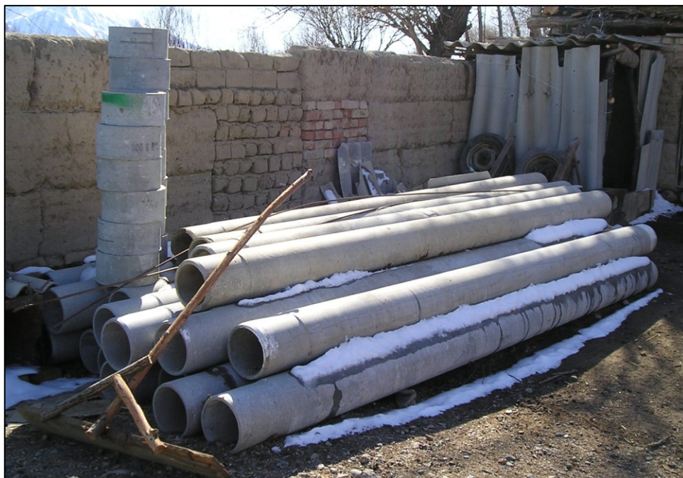
Figure 30: The asbestos pipes for the Drainage System in Kara-Suu (Photo: Topbaev, April 2011).
