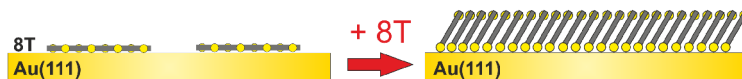
Figure 3.13: Change in the adsorption geometry from flat-lying in the submonolayer to tilted in the monolayer.
