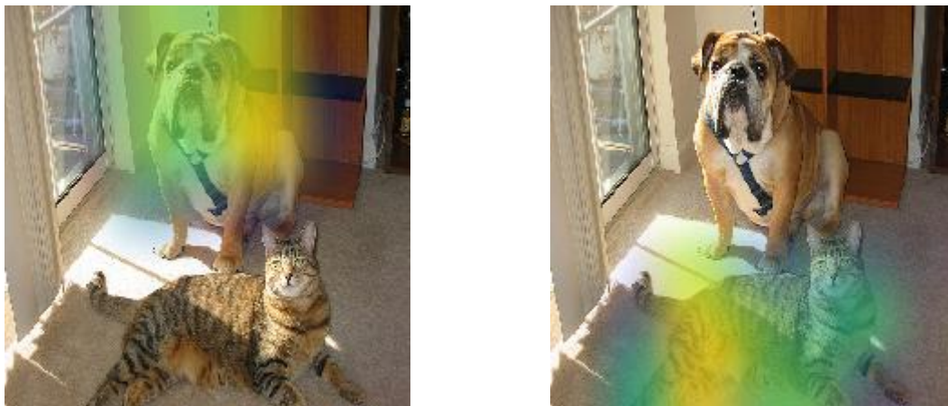
Figure 5. Example of Grad-CAM for image data - explanation for the class dog (left) and for the cat (right) (reproduced 5 ).
