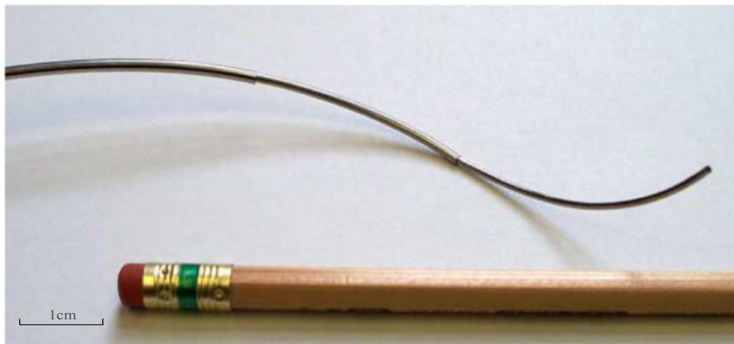
Fig. 6.1 A CTCR prototype consisting of three telescopic Nitinol tubes (adapted from (Rucker et al., 2010)).
