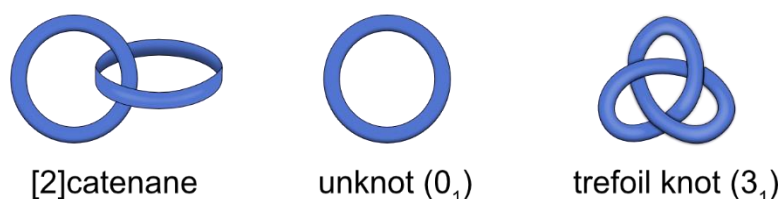
Figure 2.12: The different types of MIMs: Catenanes consist of multiple interlocked rings whilst knots are molecules with entangled conformations.
