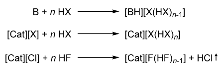
Scheme 1. Synthetic routes for the synthesis of poly(hydrogen halide) halogenates (–I).
