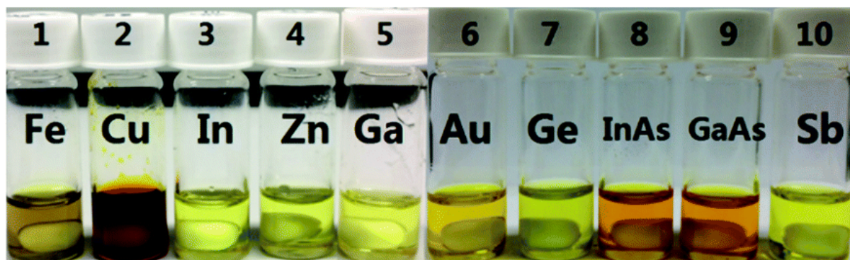
Figure 16. Metals and Alloys dissolved in [P_{444,14}][Cl_3] . [161] [P_{444,14}] = Tributyl-tetradecylphosphonium. Reproduced from Ref. [161] with permission from the Royal Society of Chemistry.
