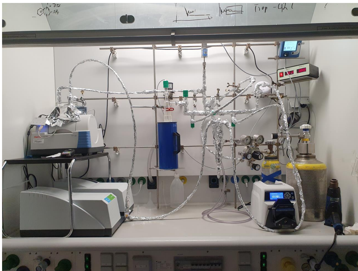
Fig. S3. Experimental setup for the investigation of the dark reaction of Cl 2 with CO. Photo Credit: Patrick Voßnacker, FU Berlin
