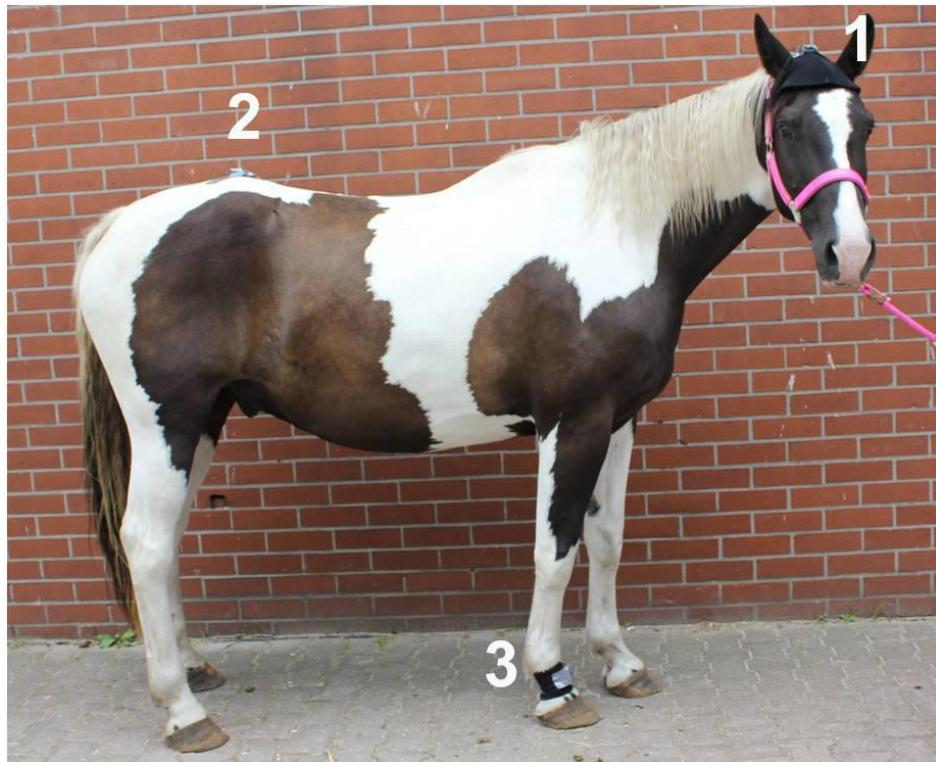
**Fig.1:** Horse instrumented with the inertial sensor system: accelerometer at the head (1), accelerometer at the pelvic (2) and gyroscope sensor for the right forelimb (3).
